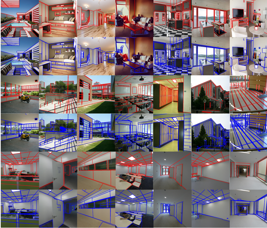
Figure 4. Qualitative evaluation of our line segment detection method. 1st row: ground truth (Wireframe); 2nd row: prediction (Wireframe); 3rd row: ground truth (York Urban); 4th row: prediction (York Urban); 5th row: ground truth (Our dataset); 6th row: prediction (Our dataset)
